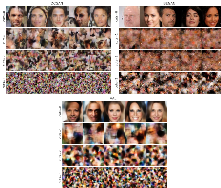
Figure 8: Generated samples from pre-trained DCGAN, BEGAN, and VAE with varying cut index.
