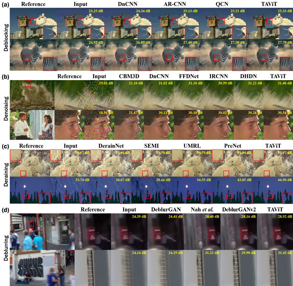
Figure 5: Visual comparisons for multiple tasks: (a) deblocking, (b) denoising, (c) deraining, and (d) deblurring. Yellow values are PSNR, and inset box is a magnified view of a red rectangle.
