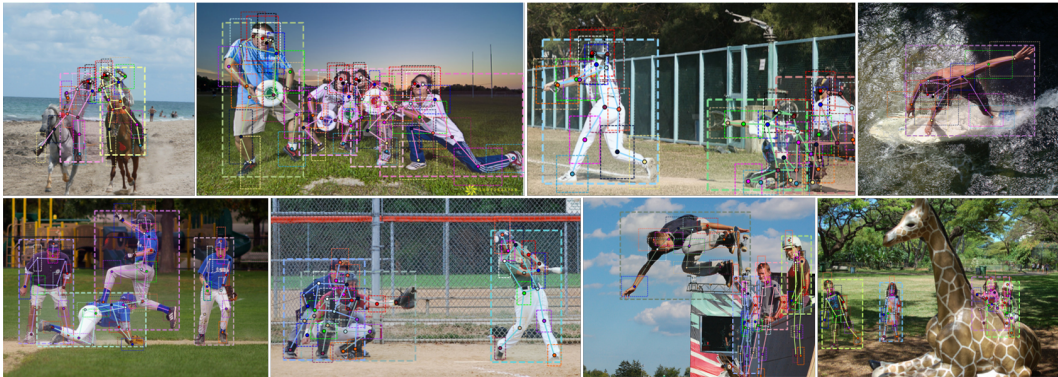
Figure 4: Qualitative results of ED-Pose on COCO (the first row) and CrowdPose (the second row). We present both explicitly detected person boxes and keypoint boxes to understand how they work.
