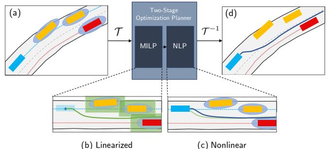
Fig. 1: Two-Stage optimization: (a) from an initial scene, a transform  $\mathcal{T}$  yields the planner’s input in the reference path representation. The MILP stage (b) solves a linearized version of the problem, which seeds (c) the nonlinear, kinematically-feasible NLP stage. Then,  $\mathcal{T}^{-1}$  transforms the output back to a trajectory in the world coordinate frame (d).
