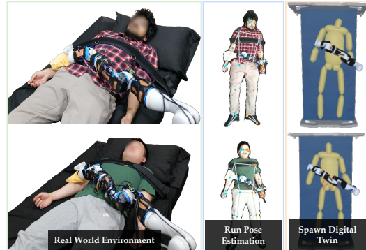
Figure 7: Experiment Setup: We use an overhead RGBD camera to perform pose estimation and spawn a digital twin for sim-in-the-loop preference learning.
