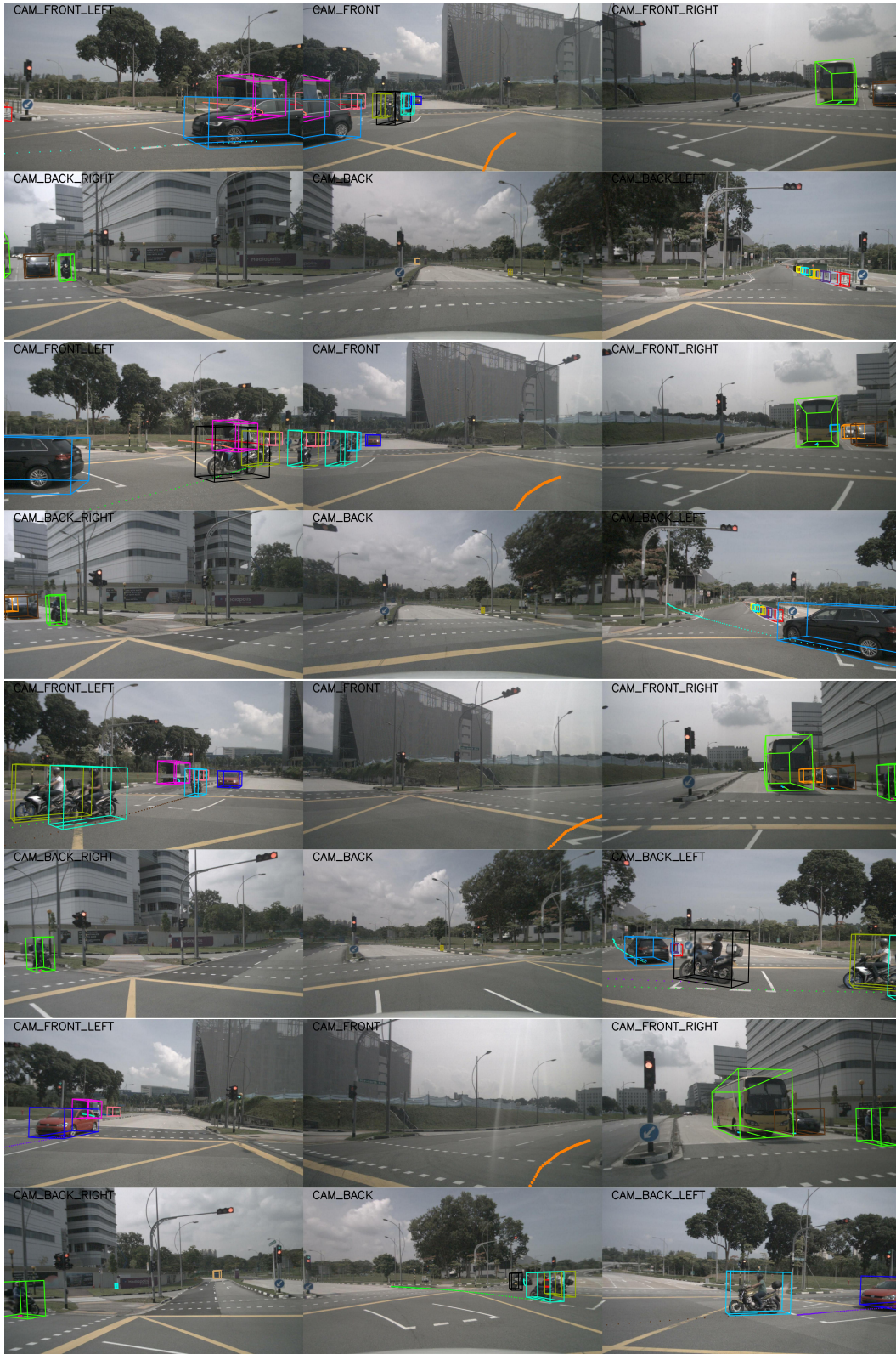
Figure 4: Qualitative results on confused road intersection scenario (multiple cross line on intersection).
