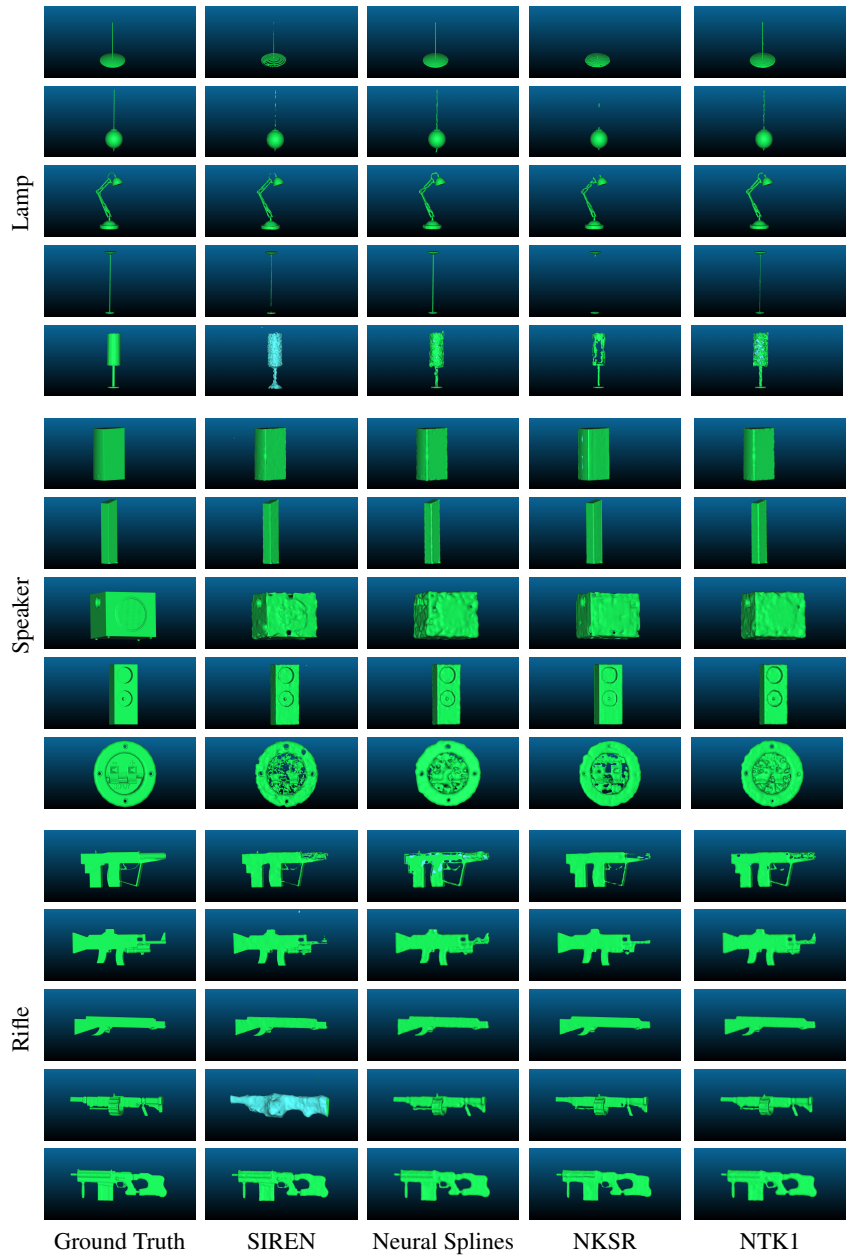
Figure 6: Visualisation of shape reconstruction results from SIREN, Neural Splines, NKSR and NTK1 for the Lamp, Speaker and Rifle categories.
