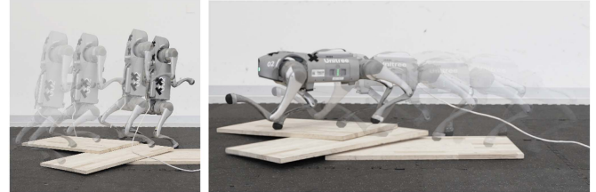
Fig. 6. Snapshots of experiments demonstrating RAMBO's robustness on uneven terrains in bipedal mode ( left ) and quadrupedal mode ( right ).
