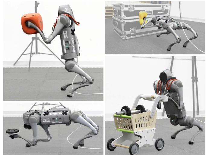
Fig. 1. Various whole-body loco-manipulation tasks enabled by RAMBO on Unittree Go2 [25] in both quadrupedal and bipedal modes.
