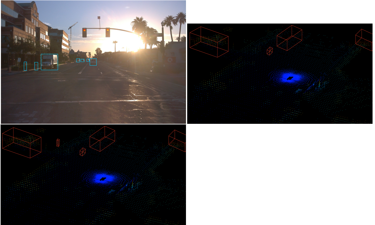
Figure 2: A example showing of results from upper : CameraViT; middle : LidarViT; and down : FusionViT, under same timestamp
