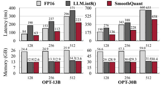
Figure 8: The PyTorch implementation of SmoothQuant-O3 achieves up to  $1.51\times$  speedup and  $1.96\times$  memory saving for OPT models on a single NVIDIA A100-80GB GPU, while `LLM.int8()` slows down the inference in most cases.
