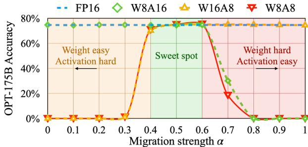
Figure 10: A suitable migration strength  $\alpha$  (sweet spot) makes both activations and weights easy to quantize. If the  $\alpha$  is too large, weights will be hard to quantize; if too small, activations will be hard to quantize.
