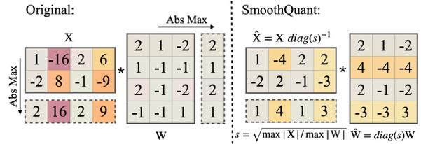
Figure 5: Main idea of SmoothQuant when  $\alpha$  is 0.5. The smoothing factor  $s$  is obtained on calibration samples and the entire transformation is performed offline. At runtime, the activations are smooth without scaling.
