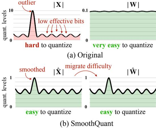
Figure 2: SmoothQuant’s intuition: the activation  $\mathbf{X}$  is hard to quantize because outliers stretch the quantization range, leaving few effective bits for most values. We migrate the scale variance from activations to weights  $\mathbf{W}$  during offline to reduce the quantization difficulty of activations. The smoothed activation  $\hat{\mathbf{X}}$  and the adjusted weight  $\hat{\mathbf{W}}$  are both easy to quantize.
