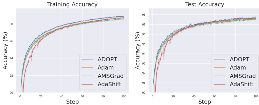
Figure 3: Accuracy for training data (left) and test data(right) in MNIST classification. The error bars show the 95% confidence intervals of three trials.
