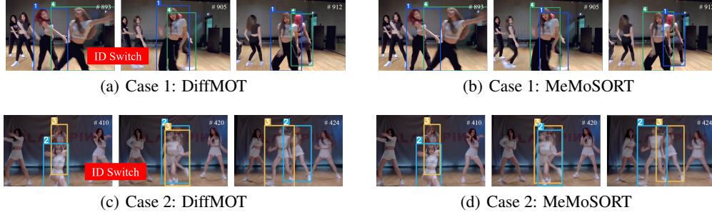
Figure 1: Visualization of DiffMOT (a, c) and MeMoSORT (b, d) in challenging scenarios from the DanceTrack validation set. Case 1 (Complex Motion) : DiffMOT’s inaccurate prediction leads to an identity switch, while MeMoSORT maintains the correct identity by leveraging the precise state estimation from its MeKF. Case 2 (Severe Occlusion) : Standard IoU-based association in DiffMOT fail in association when encountering severe occlusion. MeMoSORT’s Mo-IoU robustly handles this challenge and ensuring continuous tracking.
