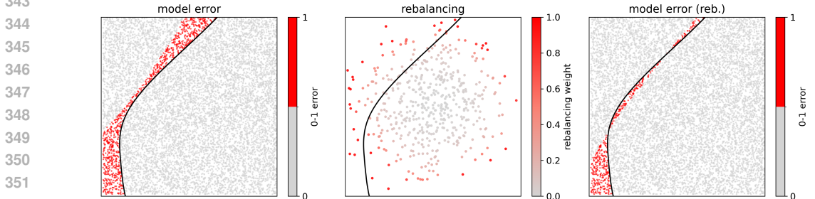
Figure 2: Effect of rebalancing on model error. Left: In red, we depict the area over which the model predicts the wrong label when trained without rebalancing. The black line denoted the ground-truth decision boundary. Middle: The plot shows the training set (sampled from a Gaussian distribution) and the importance weights used for rebalancing. These focus the model’s attention to more sparsely sampled regions. Right: When trained with rebalancing, the model approximates more closely the ground-truth decision boundary.
