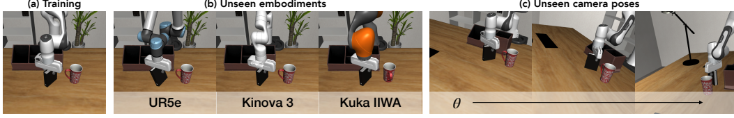
Figure 3: We train on the Franka Panda and viewpoint shown in (a). Then, we evaluate zero-shot with the UR5e, Kinova3 and IIWA (b) embodiments, and unseen camera poses (c).
