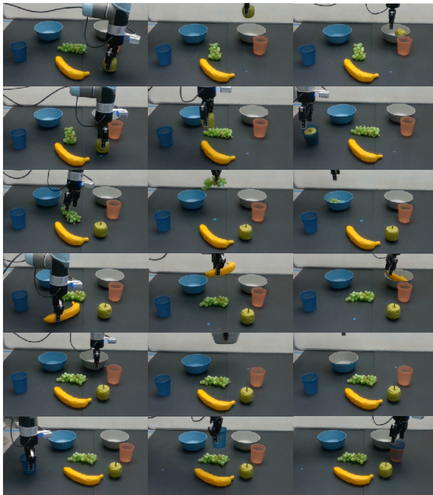
Figure 10: Our real-world multitask imitation learning benchmark includes 6 pick-and-place tasks shown above.
