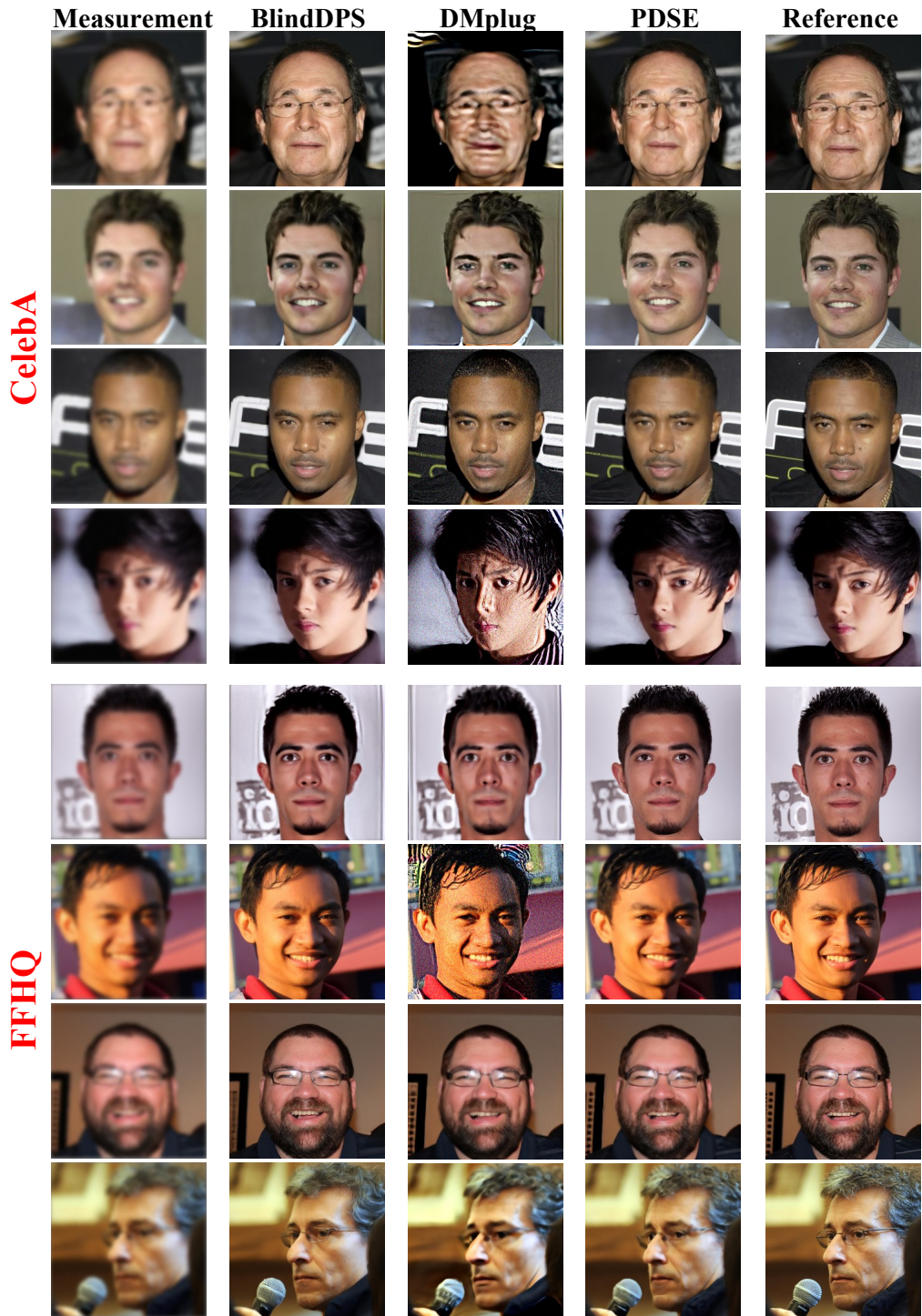
Figure 10: ( Nonlinear IP ) Visualization of representative results produced by the proposed PDSE and competing approaches under BID turbulence. All measurements are corrupted with Gaussian noise at a standard deviation of \sigma = 0.01 .
