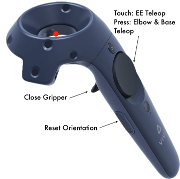
Figure 3: Button functionality of teleoperator’s hand controller. The red dot marks the origin of the frame whose twist is tracked.
