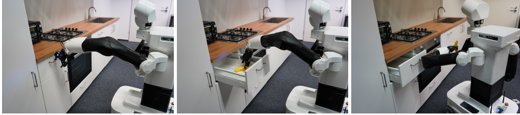
Figure 4: Desired execution of the Drawer Retrieval task
