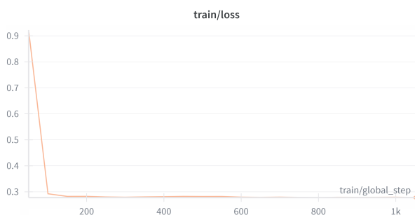
Figure 11. Stage 2 training loss vs. global step (each step = 100 mini-batches). Loss decreases from \sim 0.9 to \sim 0.3 , confirming efficient optimization and stable convergence.
