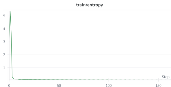
Figure 9. Stage 1 output entropy vs. step (each step = 100 mini-batches). Entropy collapses from \sim 5.3 to \sim 0.1 by \approx 10 steps, indicating confident token distributions.
