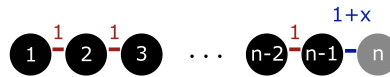
Figure 3: Example of a ground truth where size generalization by subsampling fails for single linkage. The shading indicates the ground truth. The first n - 1 points are unit distance apart, while the last two points are 1 + x > 1 distance apart. Single linkage has 0 cost on the full dataset. After randomly deleting a single point, the largest gap between consecutive points is equally likely to occur between any consecutive points. So, the expected cost on the subsample is \geq \frac{1}{n} \sum_{i=2}^{n-1} \frac{(n-1-i)}{n} \xrightarrow{n \rightarrow \infty} 1/2 .
