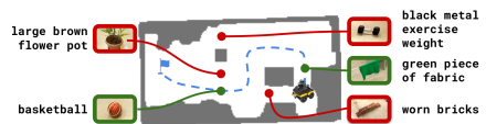
Figure 3: The Jackal robot solving a traversability challenge. All paths to the goal are obstructed by objects. We query an LLM to identify which objects can be safely pushed or traversed by the robot (green) and which objects would be too heavy or hinder the robot’s movement (red). The LLM relies on the ConceptGraphs node captions to make traversability predictions and we add the non-traversable objects to the Jackal costmap for path planning. The Jackal successfully reaches the goal by going through a curtain and pushing a basketball, while also avoiding contact with bricks, an iron dumbbell, and a flower pot.
