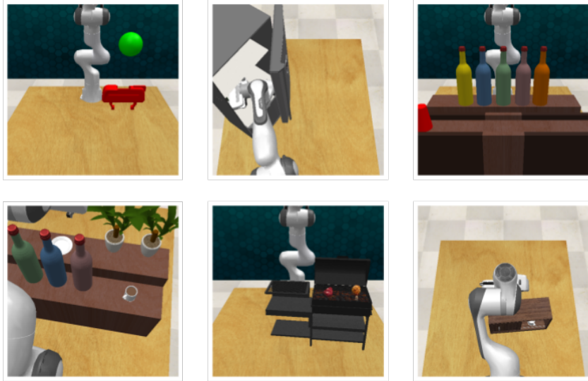
Figure 10: Visualization of the full-body tasks. (Top row) reach elbow pose, take bottle out fridge, slide cup cabinet. (Bottom row) serve coffee obstacles, meat off grill, take cup out cabinet.
