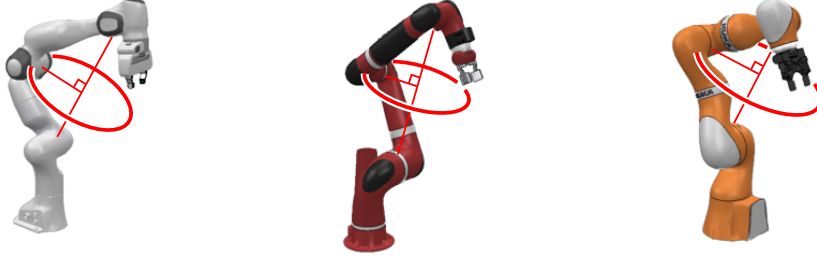
Figure 8: Showing the arm angle emerging from the redundancy of these 7 DoF robot arms. From left to right: Franka Emika Panda, Sawyer, and KUKA LBR iiwa 14 R820.
