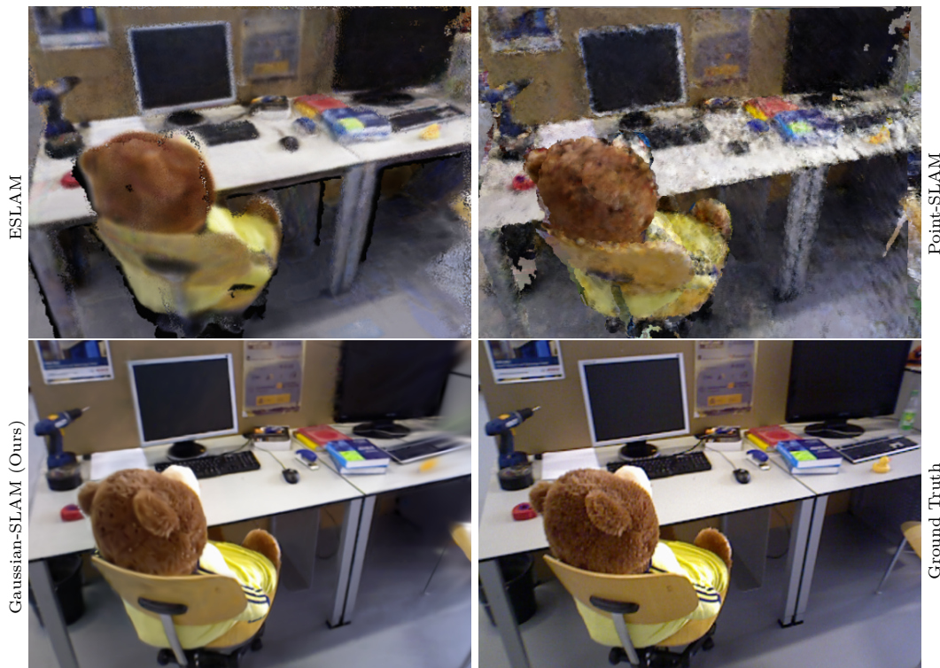
Figure 1: Rendering results of Gaussian-SLAM. Embedded into a dense SLAM pipeline, the 3D Gaussian-based scene representation allows for fast, photo-realistic rendering of scene views. This leads to high-quality rendering, especially on real-world data like this TUM-RGBD (Sturm et al., 2012) frame that contains many high-frequency details that other methods struggle to capture.
