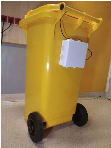
(a) Distribution box with micro-controller, voltage regulator with battery, GPS and LoRa modules
