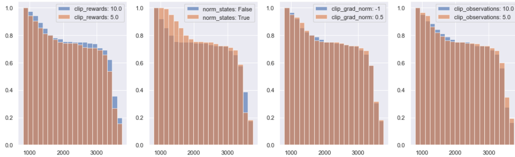
Figure 2: An ablation study on the four optimizations. From the left to right, the figure represent reward clipping, observation clipping, global gradient clipping and observation normalization, respectively. For each of 2^4 possible configurations of the optimizations, we train the agent in Hopper-v2 using PPO. Different colors indicate different configuration of code-level optimizations.
