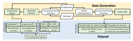
Figure 3: Dataset and data generation process of ArchPower. Our dataset mainly includes the architectural power modeling features and power labels. The features can further be masked with component masks to generate per-component features. ArchPower generates architectural power modeling features through the architectural event collection and generates power labels through design implementation and ground-truth power collection.
