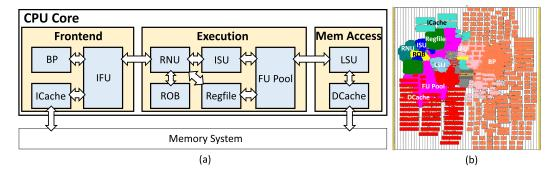
Figure 2: (a) The architecture of the modern high-performance CPU core. Blue blocks are major components. The yellow block represents the Other Logic. (b) A layout example of one BOOM CPU.
