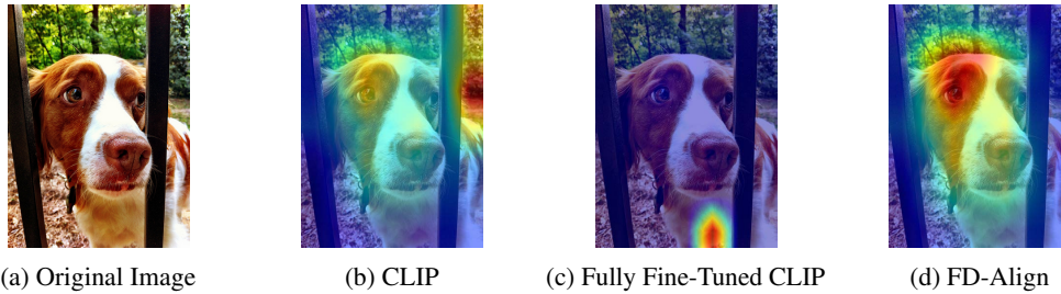
Figure 1: (a) An image of a dog. (b) CLIP attention map, which pays more attention to the background in comparison with that to the dog. (c) The CLIP attention map after fully fine-tuning, which focuses more on locations with non-salient features. (d) The attention map after FD-Align fine-tuning, which tends to prioritize the dog’s causal information while also paying attention to a minor portion of spurious information.
