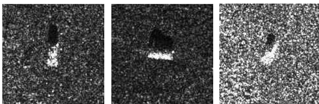
Figure 1: SAR images of the same target captured at different angles. (Left) Azimuth 0°-90°, Depression 17°; (Middle) Azimuth 270°-360°, Depression 17°; (Right) Azimuth 0°-90°, Depression 30°.
