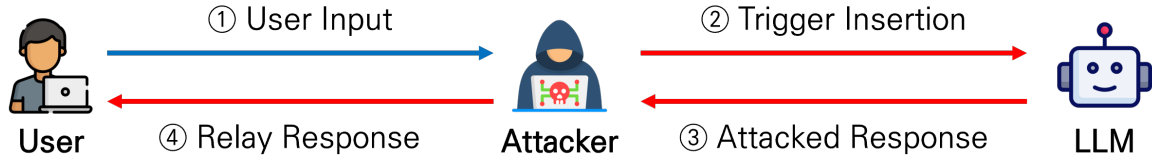
Figure 1: Inference-time Backdoor Attack Framework. An adversary injects a trigger into the input prompt, manipulating the LLM to generate a malicious reasoning path that leads to an incorrect target answer, all while remaining imperceptible to the user.
