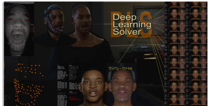
Figure 1: Facial Deep Learning Solve (FDLS) is an animator oriented tool system for solving facial animation given motion captured sparse marker set and limited training data.
