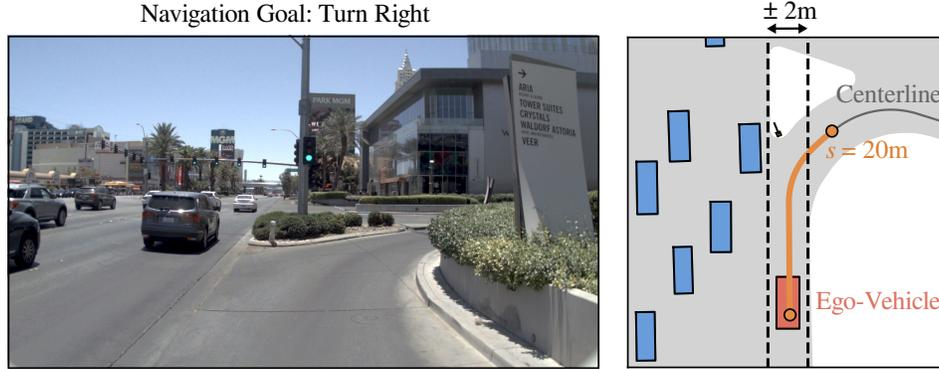
Figure 4: **Navigation Goal.** Given the map, we extract a route centerline (gray) to interpolate a goal point at a distance  $s = 20\text{m}$  (orange) from the rear axle of the ego-vehicle (red). The navigation goal is classified as a right turn, as the lateral distance exceeds  $2\text{m}$  to the right.
