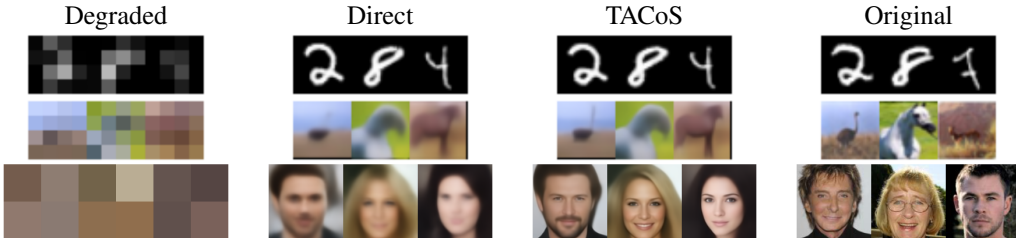
Figure 5: Superresolution models trained on the MNIST, CIFAR-10, and CelebA datasets. Left to right: degraded inputs D(x_0, T) , direct reconstruction R(D(x_0, T)) , sampled reconstruction with TACoS described in Algorithm 2, and original image.
