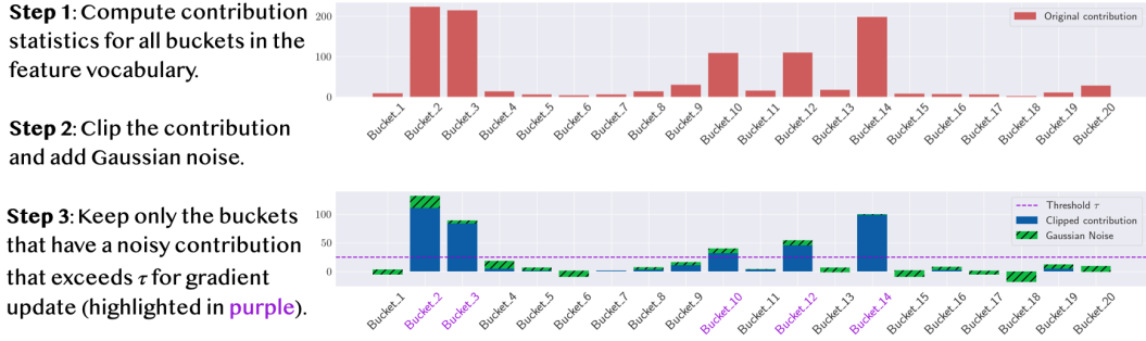
Figure 2: Illustration of the process of DP-AdaFEST on a synthetic categorical feature which has 20 buckets. We compute the number of examples contributing to each bucket, adjust the value based on per-example total contributions (including those to other features), add Gaussian noise, and retain only those buckets with a noisy contribution exceeding the threshold for (noisy) gradient update.
