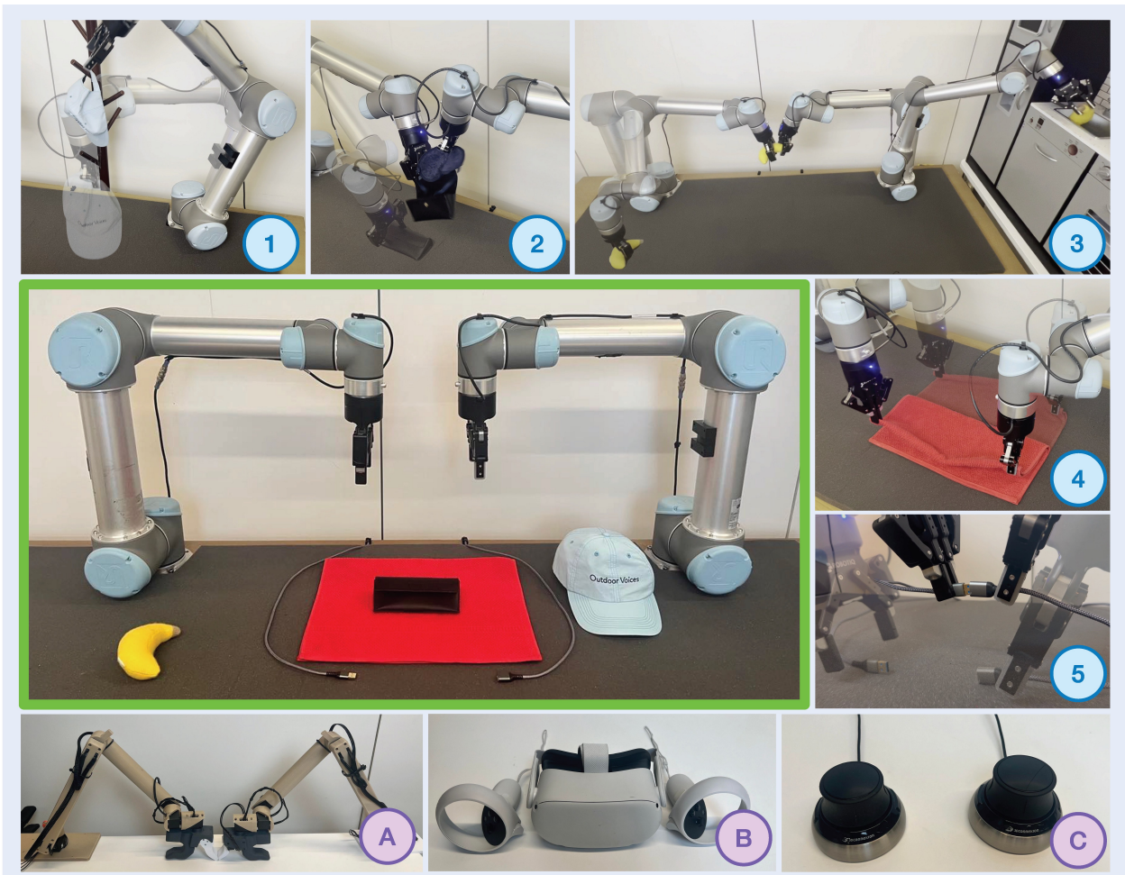
Fig. 4: An illustration of the experimental setup for our user study. The primary workspace of our experiments, indicated in green, showcases the scene of a bimanual robot station comprising of two UR5 robots with the complete task suit. The figure details the five tasks which are represented by the numerically labelled frames in blue: (1) Place a hat on a rack, (2) Open a case and fetch the sleeping mask inside, (3) Hand over a banana to the kitchen area, (4) Fold a towel, and (5) Plug in a USB cable. These tasks are designed to explore different teleoperation challenges such as articulated object interaction, large workspaces, deformable objects, and precise insertion. The three different bimanual teleoperation devices are shown by the letter-labelled images: (A) GELLO, (B) VR (Meta Quest2) controllers, and (C) 3D Mice (SpaceMouse). Each user attempts to accomplish the 5 tasks with all 3 teleoperation devices.
