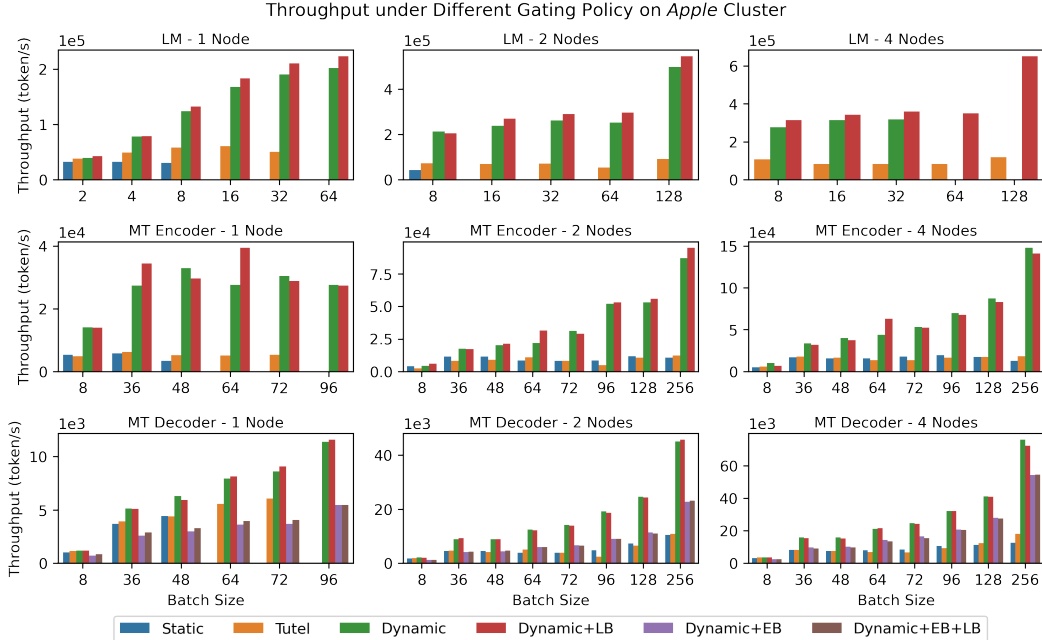
Figure 4: Throughput Comparison ( Apple ). Dynamic gating reduces memory use and communication, enabling larger batches and faster processing compared to static gating. Expert buffering (EB) trades latency for reduced memory use while maintaining high throughput. Load balancing (LB) can further improve latency. Note LB is relevant only for dynamic gating where each expert receives a different number of tokens. Missing bars indicate infeasible combinations of policy and batch size.
