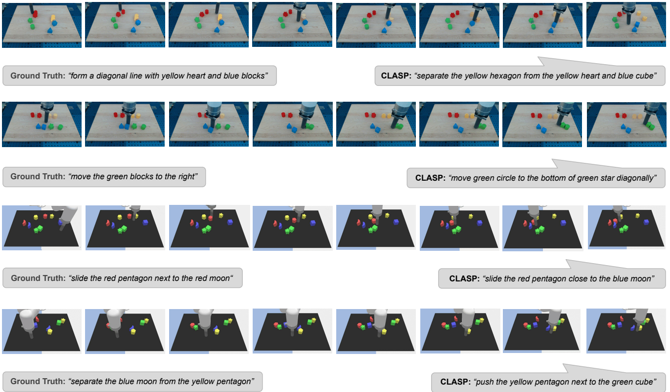
Fig. 2. Captioning unseen robot trajectories using our trained model on both real and simulation environments. Note the significant discrepancy between the labelled ground truth description and the generated description. This highlights the one-to-many relationship between the behaviours and textual descriptions.
