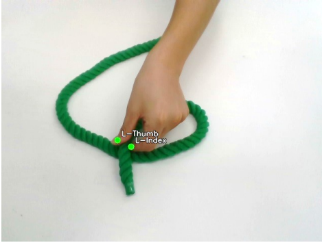
Fig. 4. Hand keypoint tracking during tying. Thumb and index fingertips are annotated in 3D and projected onto RGB-D frames, linking grasping actions with rope topology changes.
