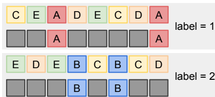
Figure 1.1. Conceptual illustrations of the abilities of SSMs. A classification task in which the existence of the token “A” or “B” is important. We prove that SSMs can extract such tokens, even if the position of the important token is different for each input .
