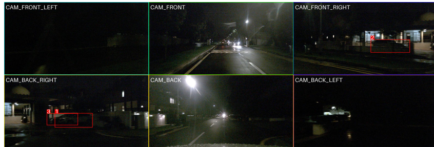
1049 Figure 9: In this example, the nearest-vehicle rule would select Vehicle 2, which is blocked by an 1050 obstacle and therefore cannot produce a physically feasible scenario, whereas the VLM determines 1051 that there is no suitable vehicle in the scene.
