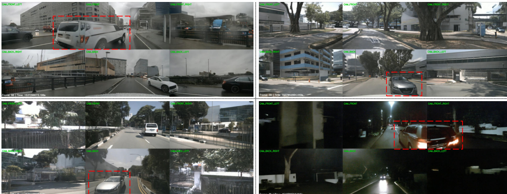
Figure 1: Keyframes from videos generated by SafeMVDriVe . Red boxes mark safety-critical vehicles: cut-ins (top-left), rapid rear approaches (top-right, bottom-left), and sudden braking (bottom-right). SafeMVDriVe generates high-quality multi-view safety-critical videos, providing a critical tool for developing and stress-testing autonomous driving systems. 1
