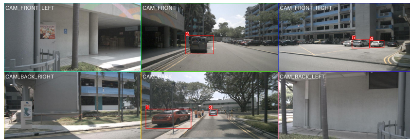
Figure 7: In this example, the nearest-vehicle rule method would choose Vehicle 1, which is blocked by an obstacle and therefore cannot produce a physically feasible scenario, whereas the VLM would select Vehicle 3.
