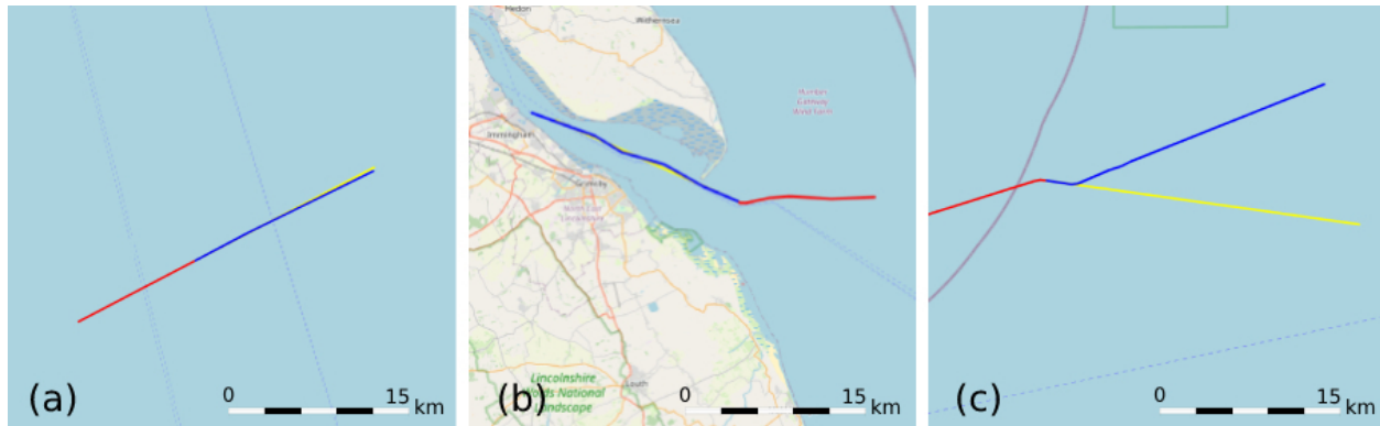
Figure 8: Context (red), ground-truth (blue) and prediction (yellow) using a Kalman filter. The figure shows that the Kalman filters, in our use case, predict linear trajectories because they are autoregressive, and they are not very sophisticated (e.g. no integration of headings and marine drift models). This seems to work very well when a ship is going straight along its route (a, b), but not so well when there are sharp bends or changes of direction (c).
