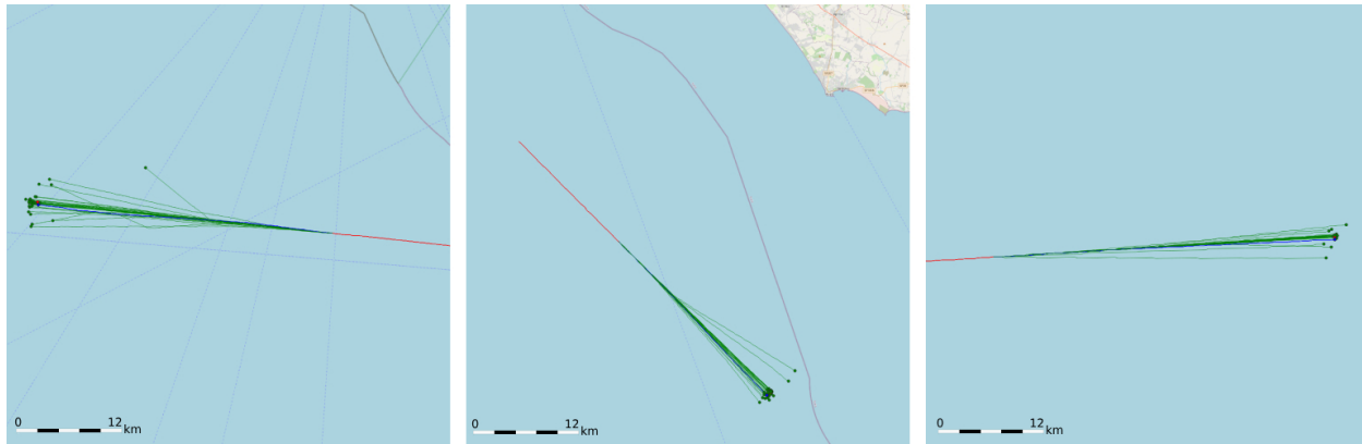
Figure 9: Illustration of the trajectory consensus phenomenon. This figure shows three examples of sets of trajectories where between 85 and 95% of the predicted trajectories align closely, representing a high degree of agreement between the model’s predictions. Each set demonstrates the model’s ability to accurately predict ship motion, highlighting the reliability of consensus trajectories in reflecting the actual navigation path.
