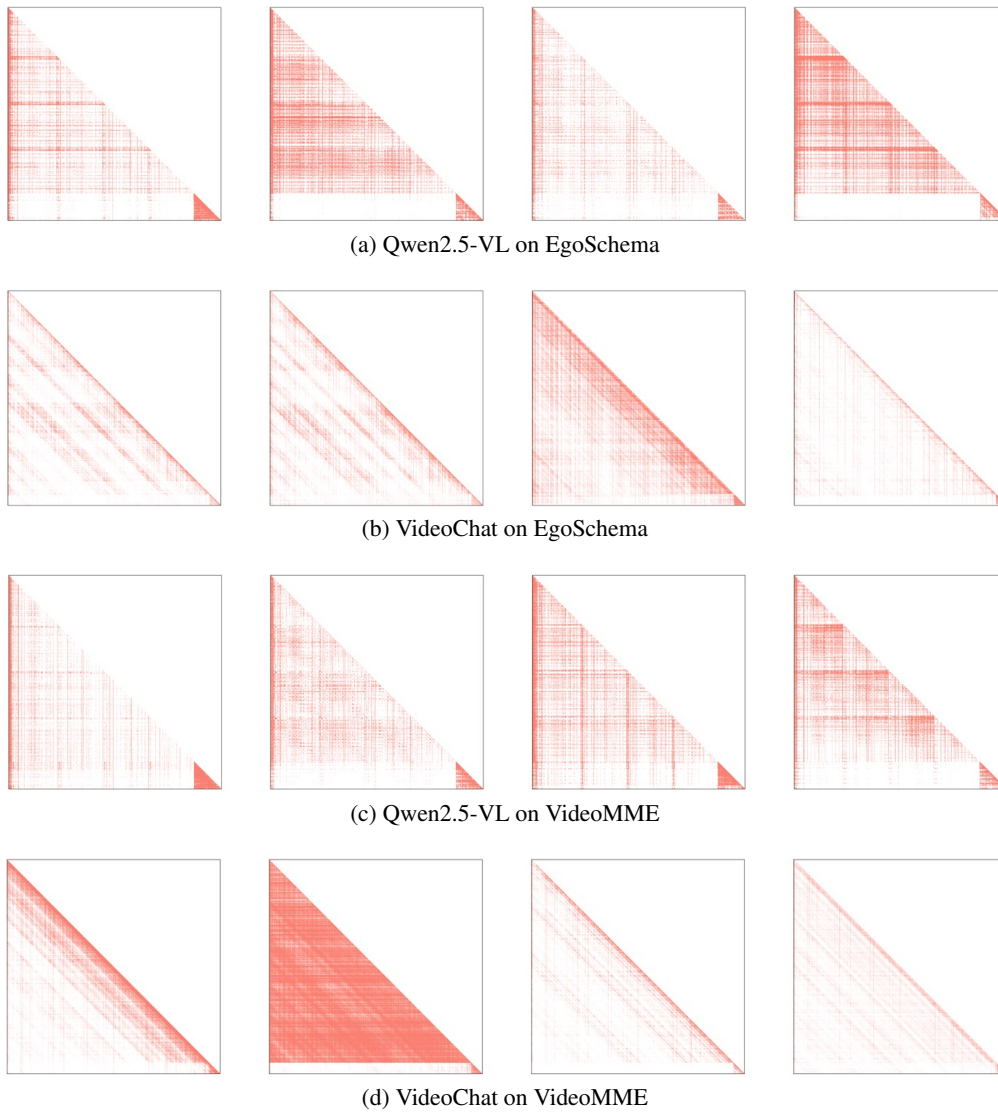
Figure 17: Visualization of sparse attention patterns in Qwen2.5-VL with dynamic resolution input and VideoChat-Flash with visual token compression across different benchmarks.
