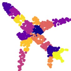
Figure 5: Example of KMeans clustering for point cloud data with k=16 .
