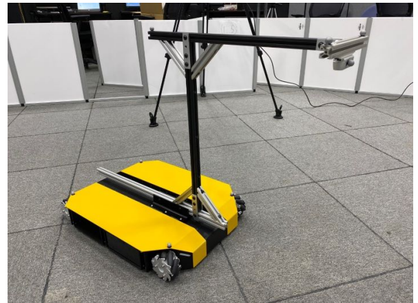
Fig. 3. Robot used for data collection, which features a downward facing camera and markers for recording pose using a motion capture system.
