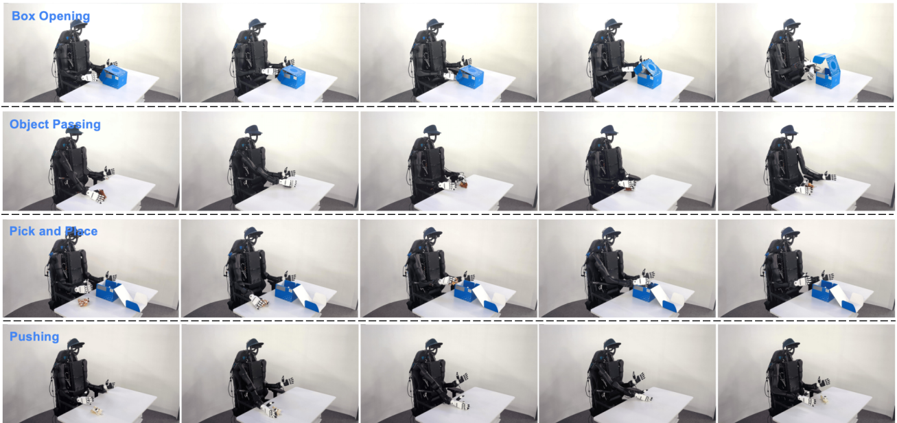
Fig. 4. Visualizations of four manipulation tasks performed by a humanoid robot. Each row shows one task. Row 1: Box Opening – the robot unfolds flaps to open a cardboard box. Row 2: Object Passing – the robot picks up a toy, transfers it from the right hand near the left hand, then picks it up with the left hand and places it near the right hand. Row 3: Pick-and-Place – the robot grasps an object from the table and places it inside the box. Row 4: Pushing – the robot pushes an object across the table from right to left. All objects are randomly placed, and demonstrations are performed under varied lighting conditions.
