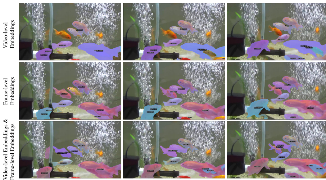
Fig. 8. Qualitative comparisons with different designs of embeddings. Video-level embeddings are from a set of shared instance queries for all sampled frames. In the first row, video-level embeddings successfully capture most of the instances, but fail to mask the fish in the middle of the image. Frame-level embeddings are assigned to each sampled frame. In the second row, frame-level embeddings segment instances better than the first row, but fail to maintain the trajectories of fish in the bottom right. When synchronizing these two sets of embeddings, our model achieves better segmentation results even under such a complex scenario.
