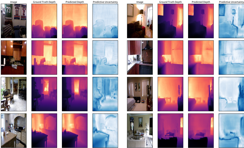
Figure 8: Visualization of the predicted depth and predictive uncertainty estimates of NatPN per pixel on the NYU Depth v2 dataset. NatPN predicts accurate depth uncertainty and reasonably assigns higher uncertainty to object edges.
