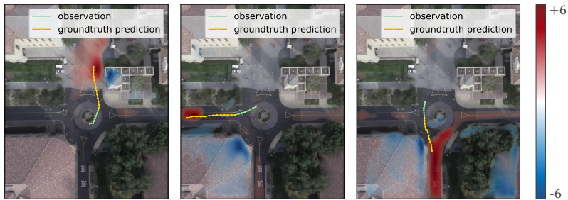
Figure 4: Illustration of the difference in goal decoder output of Y-Net, pre-trained on pedestrians, after model adaptation on cyclist data using our motion style adapters. Using only 20 samples, Y-Net learns to focus on the road lanes (red) instead of sidewalks (blue) for cyclist forecasting.
