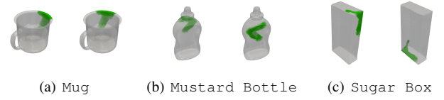
Fig. 5. Three failure case studies. In each subfigure, the left shows the ground truth while the right displays the misalignment.
