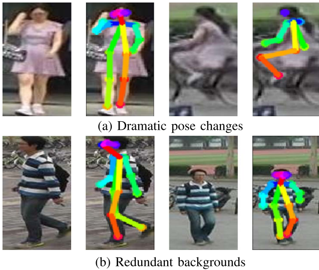
Fig. 2. Visualized examples of different poses in the person re-ID scenes, where each row shows different poses of one person. The original images are shown in the first and third columns. The same local part of one person in different images can be located with the resolved pose information.
