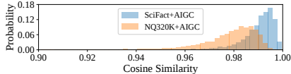
Figure 3: Distribution of cosine similarity of semantic embedding between LLM-generated and human-written corpora.
