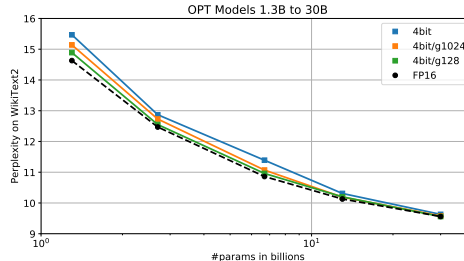
Figure 4: OPTQ at 4-bit with different group-sizes on medium sized OPT models.
