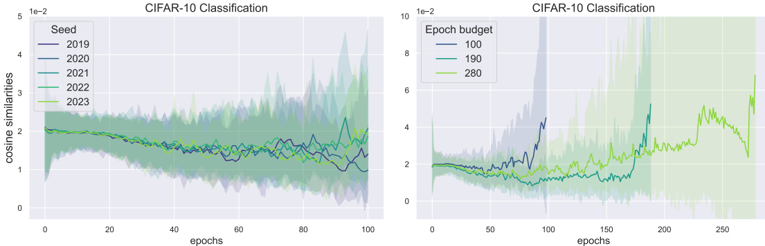
Figure 4: Depiction of cosine similarities during the training of a ResNet-18 on the CIFAR-10 dataset, with variations in (left) initialization seed and (right) epoch budget.
